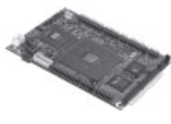
EPIA-P700 (P. 46) Pico-ITX C7®/Eden™ ULV Board with MPEG-2 & 4, WMV9 and CRT/ DVI/LVDS/DC-in
